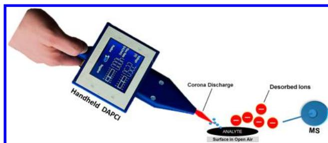
**Figure 2.** Schematic of the hand-held DAPCI experimental setup used in the analysis of nitroaromatic explosives.
